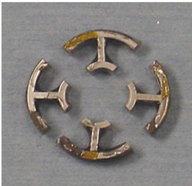
Fig. 13. Quartered thermopile prior to re-bonding and series wiring.
